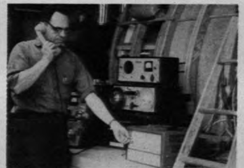
Backstage at the mock-up, sound equipment duplicates engine noise.
