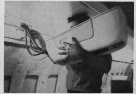
The passenger service unit is adjustable to the seat spacing, goes under the hat rack.
